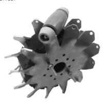
**Step 13:** Put a 10-32 Nylock Jam Nut on the end of the 10-32 x 3.25" SHCS to finish off the roller assembly. Be sure to tighten the screw enough that the rollers are spinning on the brass axles and the brass axles are **NOT** spinning on the screw. The
