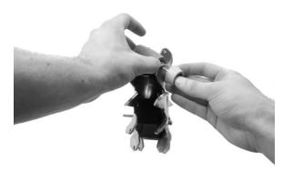
**Step 10:** Slide the Brass Outer Roller Axle onto the threads of the 10-32 x 3.25" SHCS.
